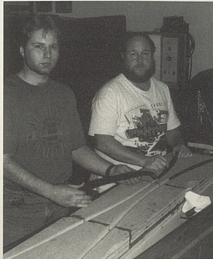
Above, John Lanzoni, left, and Matthew Lyon, right, work on the wings ribs for the Chanute glider in Rochester.
