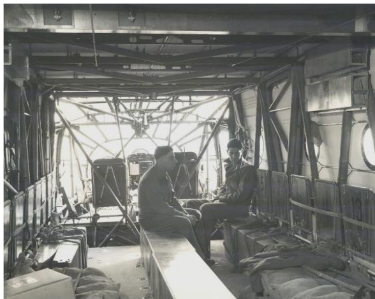
Interior of the CG-13A, showing the increased wind screen size and more capacity for transporting troops.
