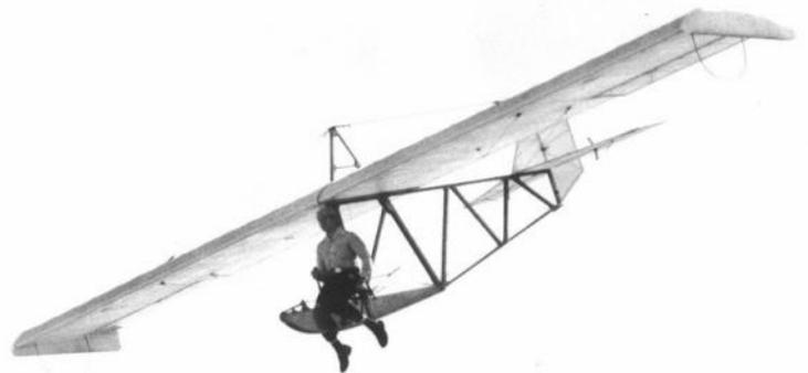
The *Rhön Ranger* consists of a simple open wooden frame fuselage with doped fabric covered section at rear, fabric covered wooden framed wing of constant cord, fabric covered wooden framed tailplane, elevators and rudder.
