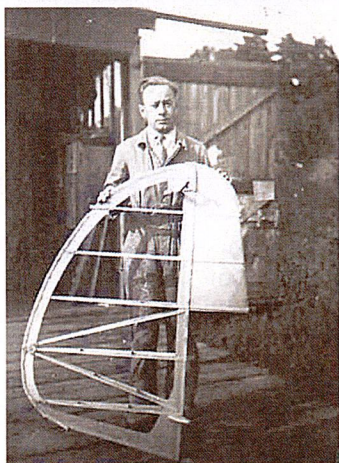
Norm with "Kirby Kite" rudder and stabilizer
