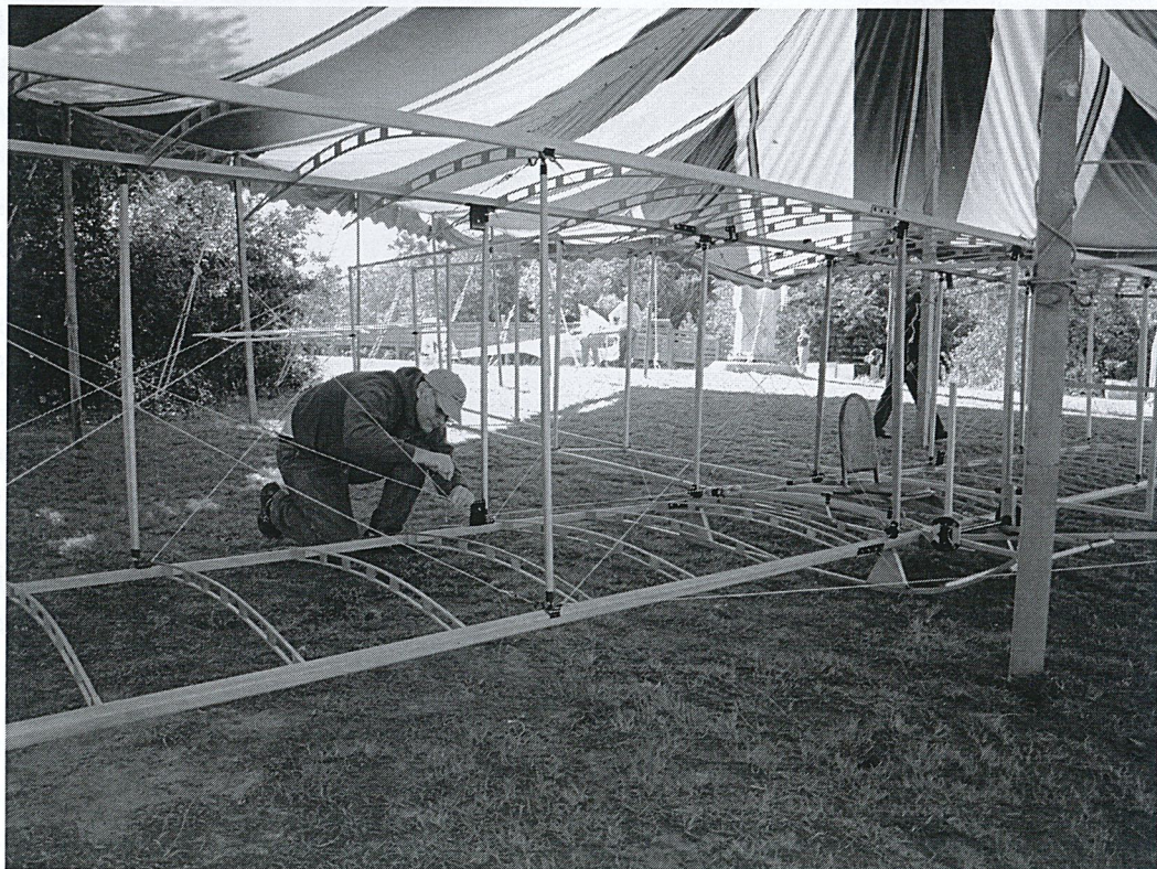
Nick Mirales is wire-wrapping the last fittings on Jimmy Dayton's Wright 1911 glider replica or "flying facsimile", with Gary van Tassel's PW-5 and several historically significant hang gliders in the background.
