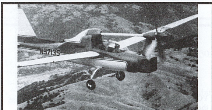
Lockheed Q-Star is a modification of the 2-32 - - used in developing the quiet observation aircraft for the military. The latest model shown above has a Wankel type engine.
