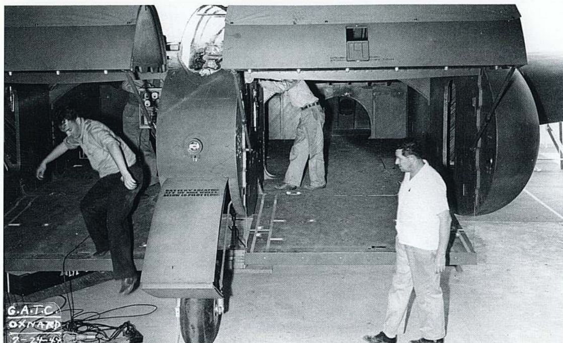
Bowlus XCG-16, showing opened clamshell leading edge, pilot and cockpit area. Stencil on nose wheel cover reads, "Battery location aft of nose wheel below co-pilot floor." Designer/Builder, William Hawley Bowlus is at lower right, others are unidentified; July 24, 1944, Oxnard, CA. (NSM Multi-media Archives)
