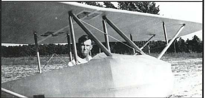
First flight of 11544 with Sanders V. Hudson Jr. in the cockpit, Aug. 10, 1932. "Was so busy getting the glider assembled, he has not shaved or combed his hair in three days." Empty 208 lbs., gross 393 lbs - L/D approx. 12 to 1 - spars, longerons, ribs, white pine.
