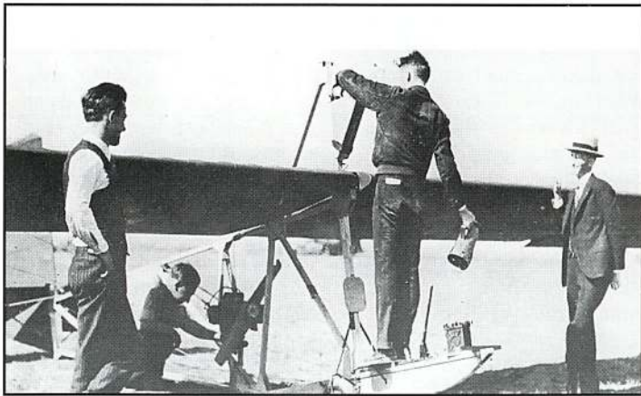
1930 Cessna CPG-1, Experimental. A modified CG-2 with a 10 1/2 hp Cleone engine. (Ibid.)
