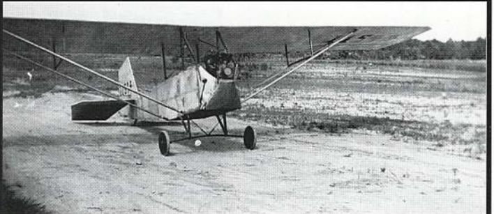
Glider 11544 after conversion to motorglider Summer 1934, Durham Airport. "Climb 40 ft. per minute in still air - 1,000 ft. density altitude on 8.59 gross horsepower. 11544 was thought to have the lowest hp for any flight ever from dirt airport and roads in the southeast U.S."
