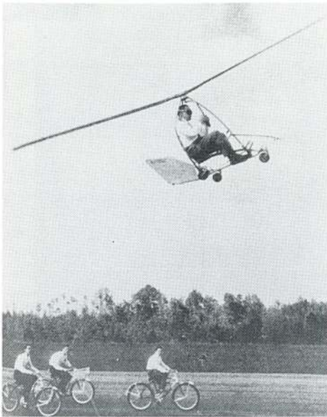
Left, the Bensen single-place gyro glider on tow, with bicycle observers following, from a May 24, 1954 Life Magazine story. Above - Bensen B-8W Hydro-Glider with streamlined 9 foot floats. Right - Bensen Model B-8 2-place Gyro-Glider (From NSM Multi-Media- Archives.)
