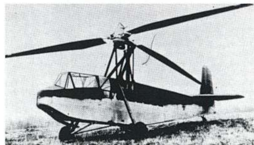
The Focke-Achgelis-Fa255- A converted DFS 230 Assault glider, minus wings, plus helicopter ro- tor, for short field landing.
