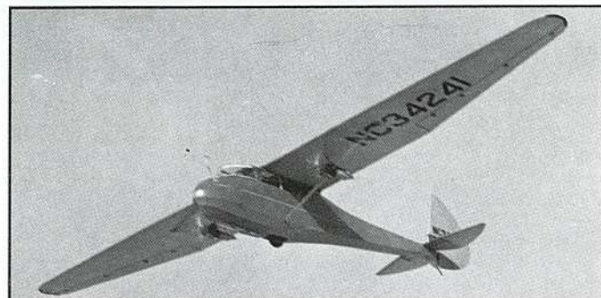
A Cinema powered glider, 1944, with dual 2 cycle 6 h.p. engines and contra-rotating props.
