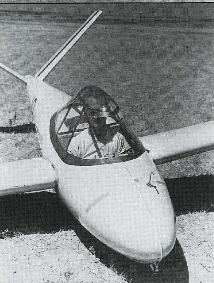
The original concept of the Prue 160 ("160" for its empty weight), with full floating controls, Rosamond Dry Lake, CA, 1946. (Irving Prue photo)
