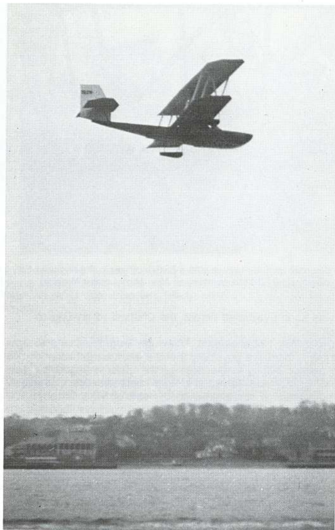
First test flight of the Peel Two-Place Glider Boat, by Richard Atwater in 1930 at College Point, Long Island, NY. The single hull biplane was based on a Curtiss hydroplane design. It had a glide angle of 15 to 1 and landed at 19 miles per hour. (Photo from the NSM multi-media collection)
