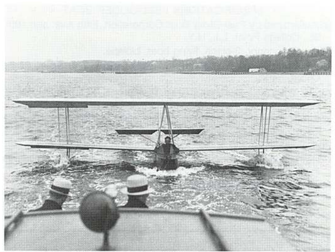
1930, College Point, Long Island, NY. Richard Atwater being pulled out to a launching position, where he would be handed a towline with a bridle that was secured by latches on either side of the Peel glider's bow. Power boat speed for the launch was about 20 miles per hour. (Photo from the NSM multi-media collection)
