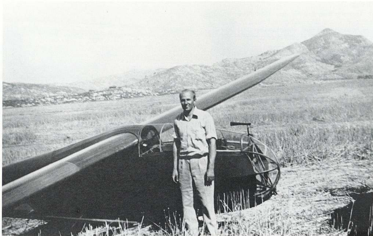
Robinson and his Robin #4 sailplane, showing its transparent nose, 1938. John Robinson Photo
