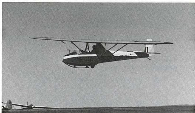
Jan Scott's Slingsby Cadet Model III, T-31, two place former RAF Trainer on final during the Vintage Sailplane Regatta, May 27 & 28 at Harris Hill. The T-31 has a glide ratio of about 17 to 1 and is the only one in the United States.
