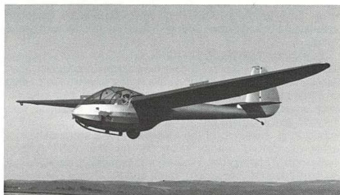
Pilot Bruce Barrett eases the WW II Pratt Read TG-32 in during the Vintage Sailplane Regatta. This ship is distinct in that it was the only training sailplane with side-by-side seating and was the only training glider designed for the Navy. That's the Loon from Jeff MacNelly's cartoon, "Shoe," painted on the P-R's nose.
