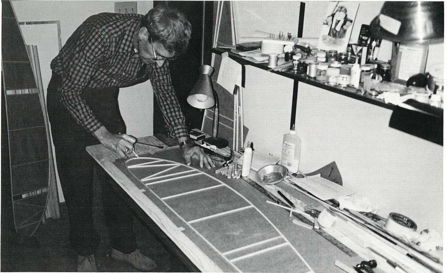
Replica of the 1929 rib used on the Bowlus Model SP-1, "Paper Wing" sailplane. Trimming paper from the edge of wing rib after first side has been completed.
