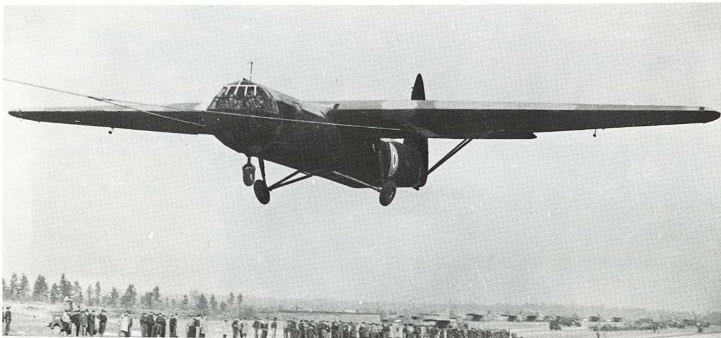
Pick up of a British Horsa glider. Note bifurcated tow yoke.
