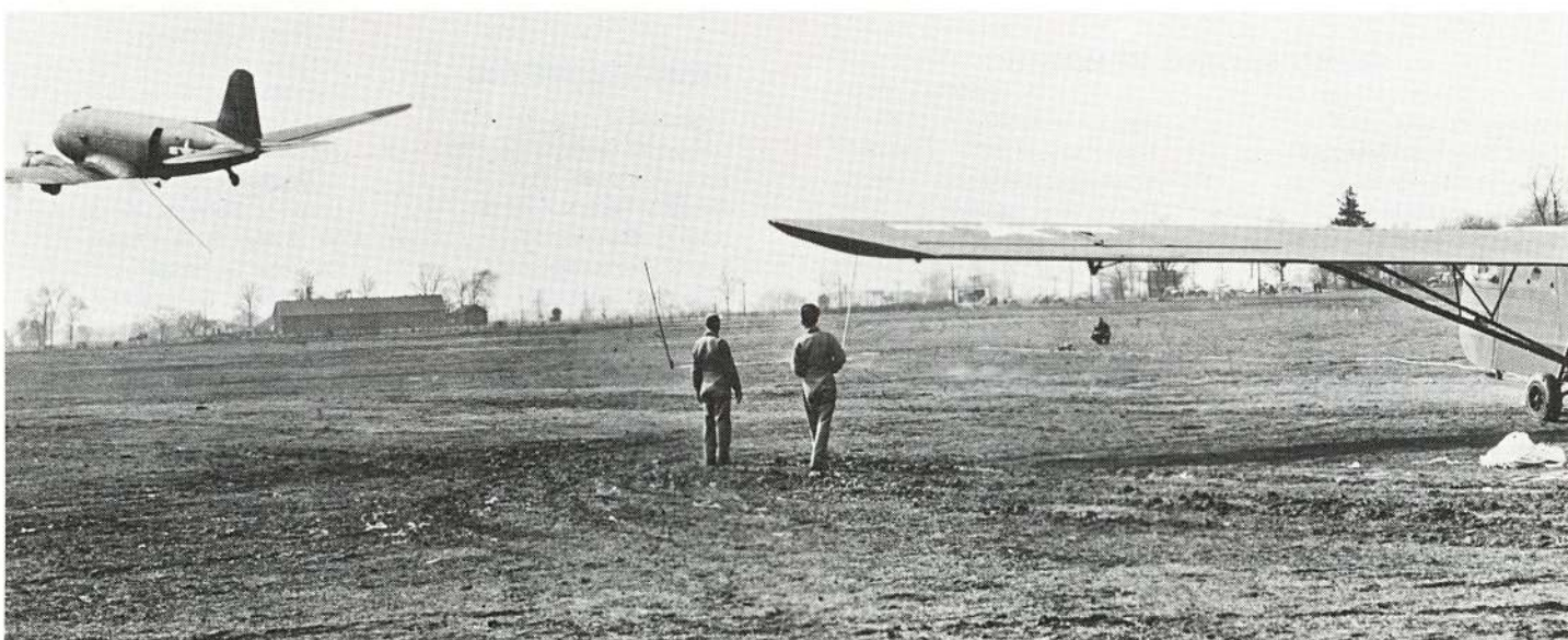
Clothesline pick up of a CG-4A by a C-47. The C-47 has just received towline loop from station poles. The tension is not yet on the CG-4A.
