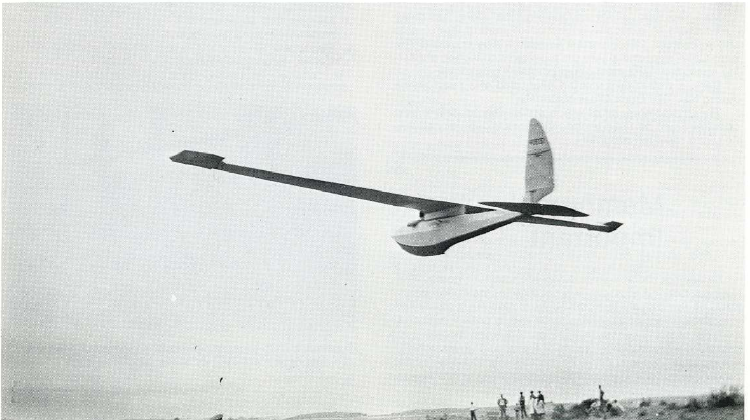
H. Bowlus's Albatross No. 16 at the first glider meet, July 4, 1929, Pacific Beach, California — Span - 44 feet, AR-11, and
