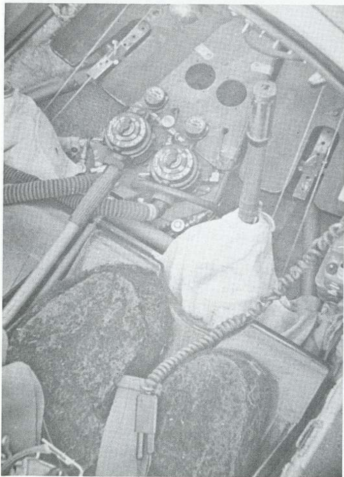
The Pratt Read's oxygen installation.
