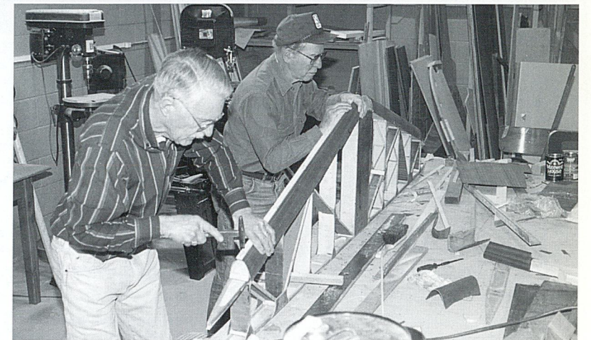
Above, NSM Volunteers Erwin Jones (left) and Dale Gustin put some loving repair into the Wolf's stabilizer.
