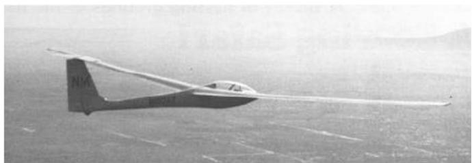
Perhaps his most well-known design was the Applebay *Zuni* and the later refined *Zuni II*. These sailplanes are single-seat, water-ballasted designs intended to compete with the European fiberglass gliders in the 15-Meter class. The *Zuni* was designed in 1975 with particular attention to achieving laminar flow. Using the classic pod and boom
