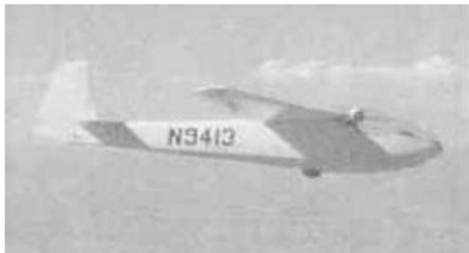
many varied and successful sailplane designs. The GA-II *Chiracahua* is a high-wing, single-seat standard class glider which first flew in 1970 after 11 years of work. This craft had an empty weight of 590 lbs and gross weight 819 lbs. The 15-Meter (49 ft 3 in) wing had a Göttingen 549 airfoil and an aspect ratio of 16.2.
