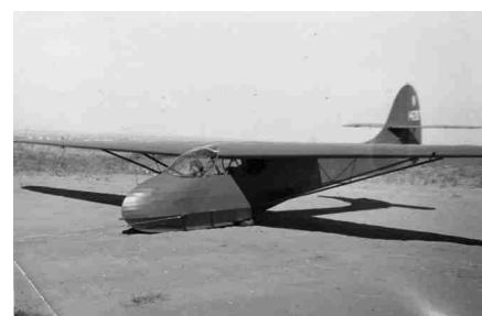
Handles on side serve as tow hooks for "Y" shaped tow rope
