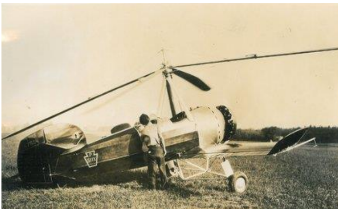
The Autogyro 1930 with 110hp Warner, built by Alfaro under contract from Pitcairn, and was also known as the Pitcairn-Cierva PCA-2-30 .
