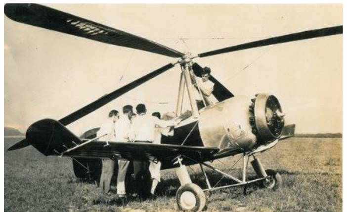
The Autogyro 1930 with 110hp Warner, built by Alfaro under contract from Pitcairn, and was also known as the Pitcairn-Cierva PCA-2-30 .
