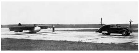
Franklin PS-2 training glider is about to be towed aloft by the specially modified car in front.
