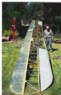
Schweizer 1-7 assembled in Cannon's backyard in Palo Alto, CA before covering.
