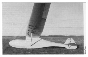
This sailplane, the Schultz Nucleon, was built in 1954 and had a span of 46 feet with aspect ratio of 16 utilizing an NACA airfoil NACA 65(2)-415, 64(1)-A212. Empty weight was 345 lbs with gross weight 535 lbs. The structure was single strut braced all-wood wings, steel tube/fabric wings and braced tail. L/D estimated at 22 (47 mph) and minimum sink 3.3 fps at 43 mph. The wing was built of
