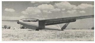
Next followed the Prue 215. Again it was all-metal, flush riveted and included a reclining cockpit, an external airfoil flap and a retracting landing wheel. Irv chose aluminum as the material for this and his succeeding designs.
