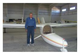
The Applebay *Zia* is a single-seat, high-wing, twinboom, pusher motor glider originally designed for the 1982 Sailplane Homebuilders Association Homebuilt Sailplane Design Contest but withdrawn in order to make further changes. The wing span is 46 feet, aspect ratio 18, airfoil Wortmann FX 66-197, empty weight 400 lbs, gross weight 650 lbs. It carries 4 gallons of fuel and has a Rotax 277, 28 hp engine. Max glide ratio is 25.
